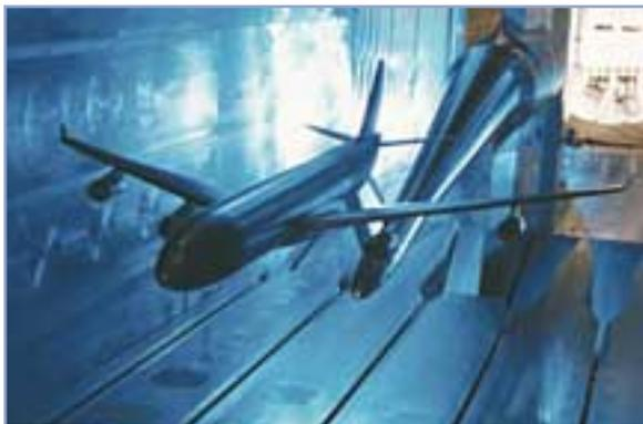
Figure 4: Aircraft Model in the ETW Test Section
