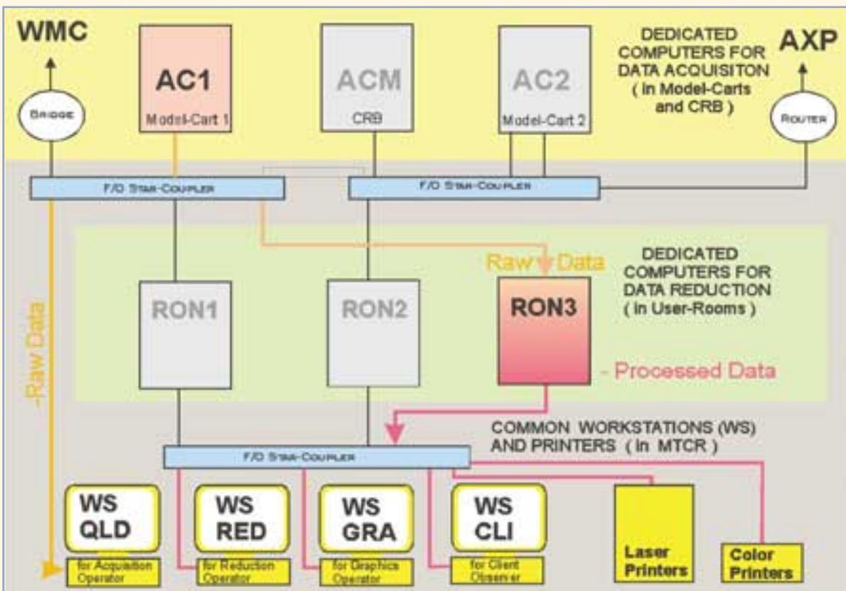
Figure 23: Model Data Acquisition Network Schematic
