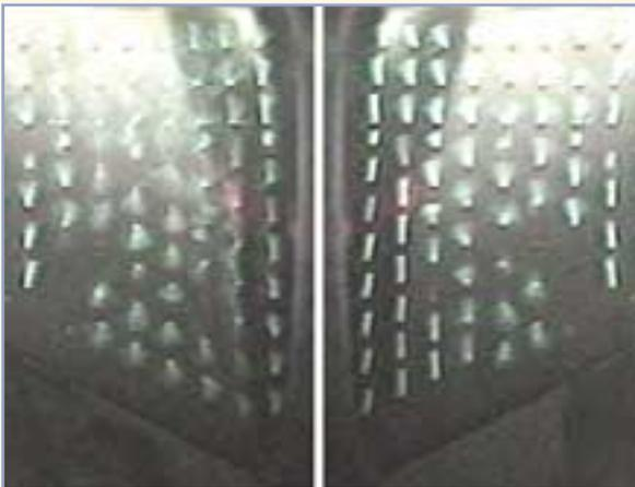
Figure 19: Flow Details Indicated by Minitufts
