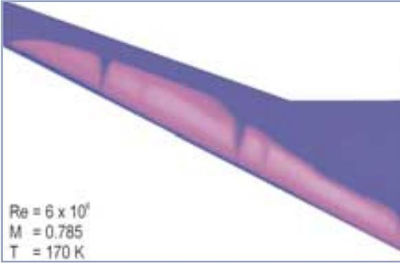
Figure 18: Visualization of Boundary Layer Details by Temperature Sensitive Paint
