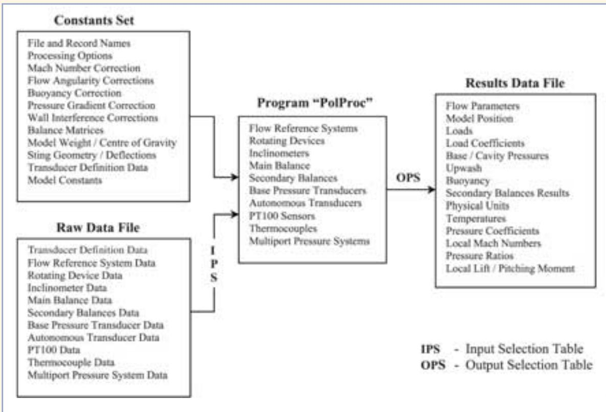
Figure 24: Data Reduction Schematic
