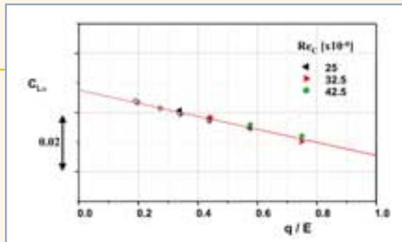
Figure 13: Aeroelastic Effects on Lift Curve Slope
