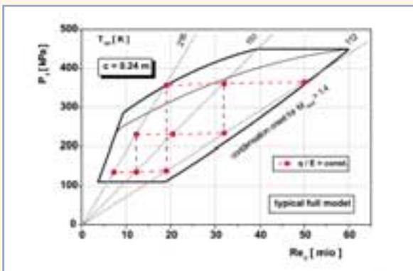
Figure 11: Operating Envelope for  $q/E$  testing
