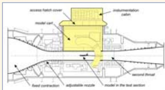
Figure 5: Test Section and Plenum
