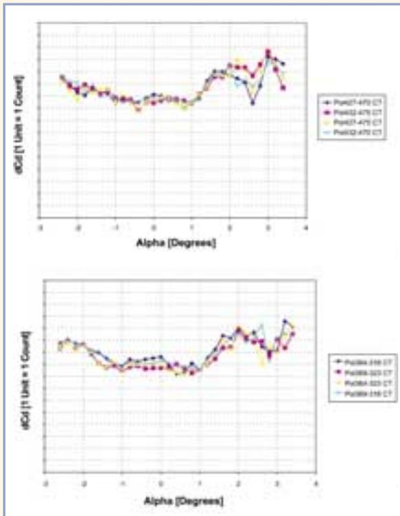
Figure 22: Drag Increments Measured with the ETSR Technique
