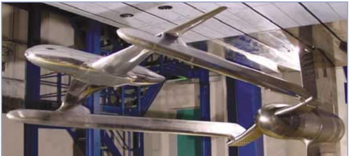
Figure 21: Enhanced Twin Sting Rig
