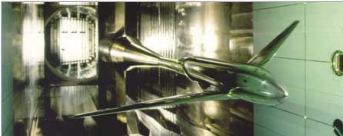
Figure 25: Model on Straight Sting in Test Section
