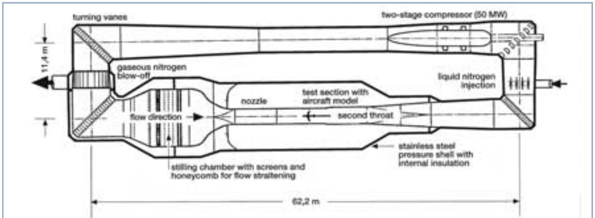
Figure 3: Aerodynamic Circuit
