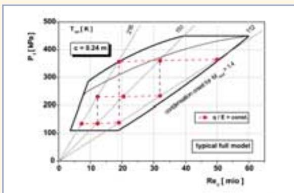
Figure 11: Operating Envelope for  $q/E$  testing
