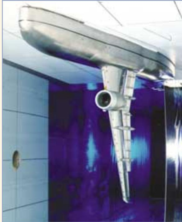
Figure 26: Half Model in High Lift Configuration
