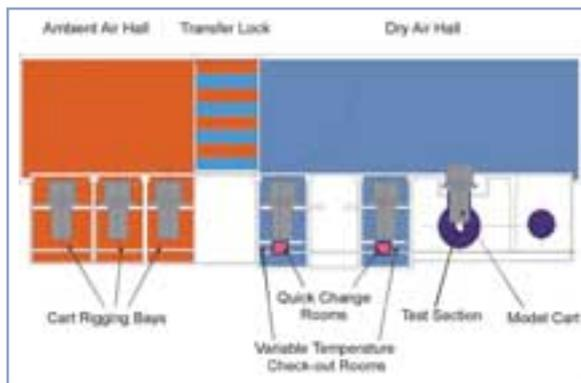
Figure 7: Section through Transfer Hall
