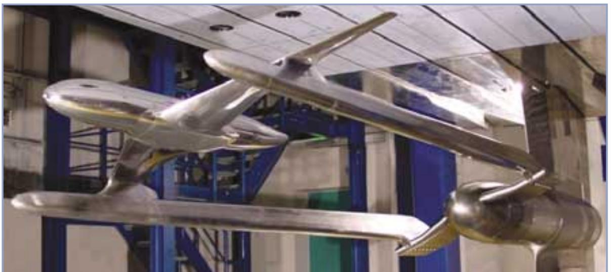
Figure 21: Enhanced Twin Sting Rig
