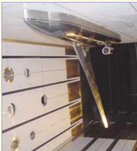
Figure 6: A Half Model in the ETW Test Section
