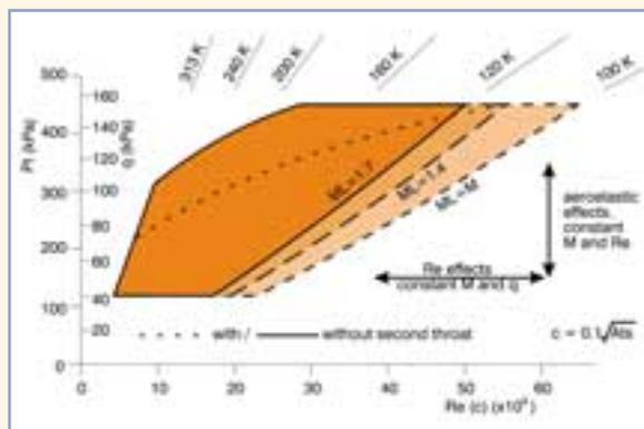
Figure 2: Example for Test Trajectories for Reynolds Number and Aeroelastic Effects, Holding Mach Number Constant ( $M=0.9$ )
