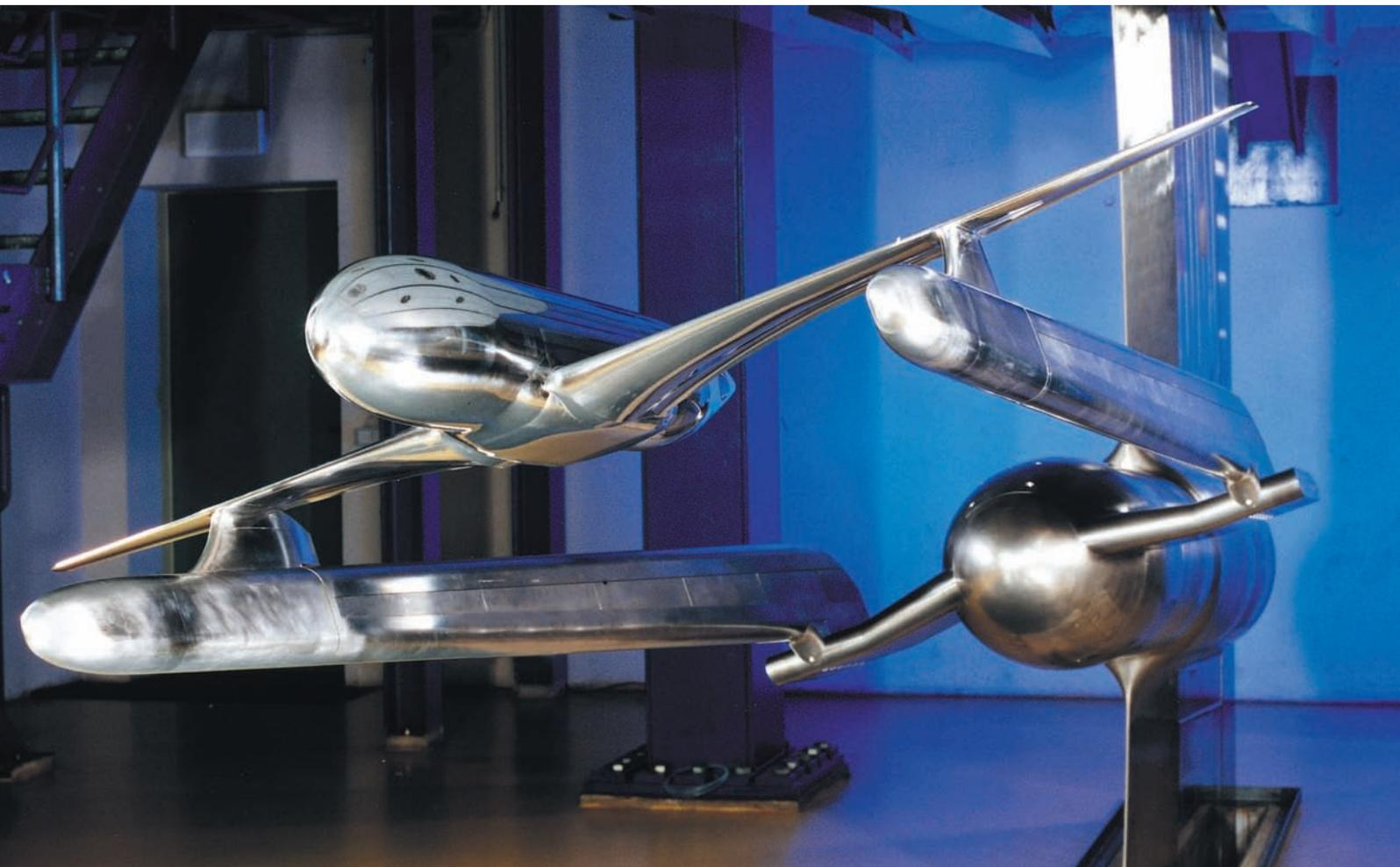
The forces and moments exerted by the flow on the model are measured with high precision strain gauge balances.
