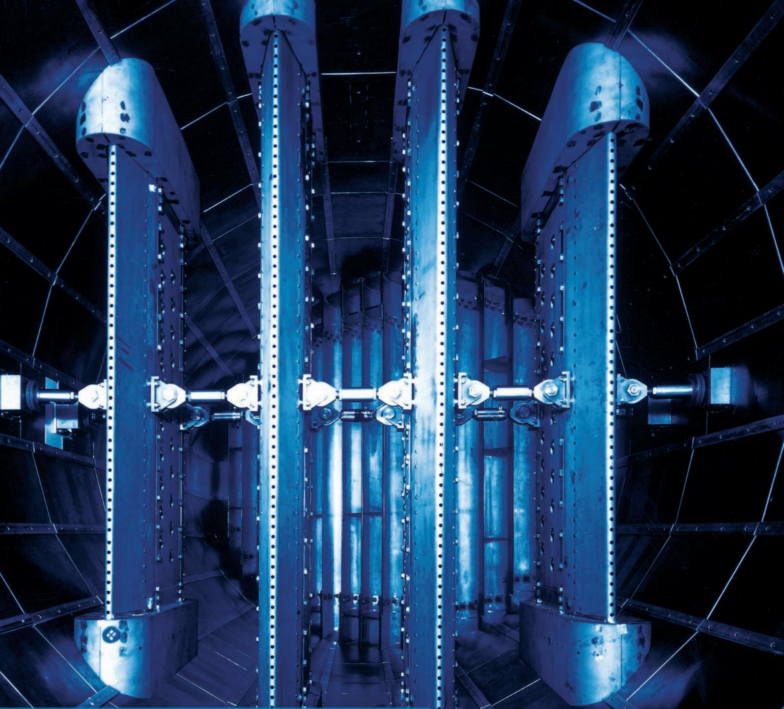
Liquid nitrogen is sprayed into the flow through 240 nozzles distributed over the four vertically mounted injection rakes
