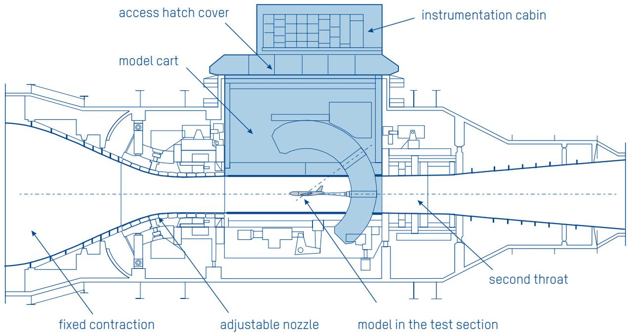
Model Cart with model in the test section
