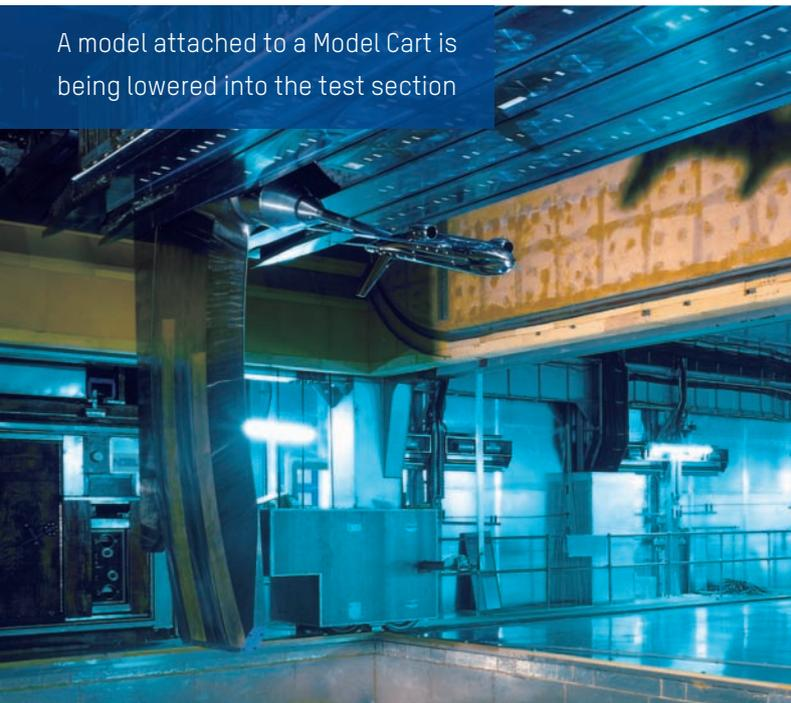
A model attached to a Model Cart is being lowered into the test section
