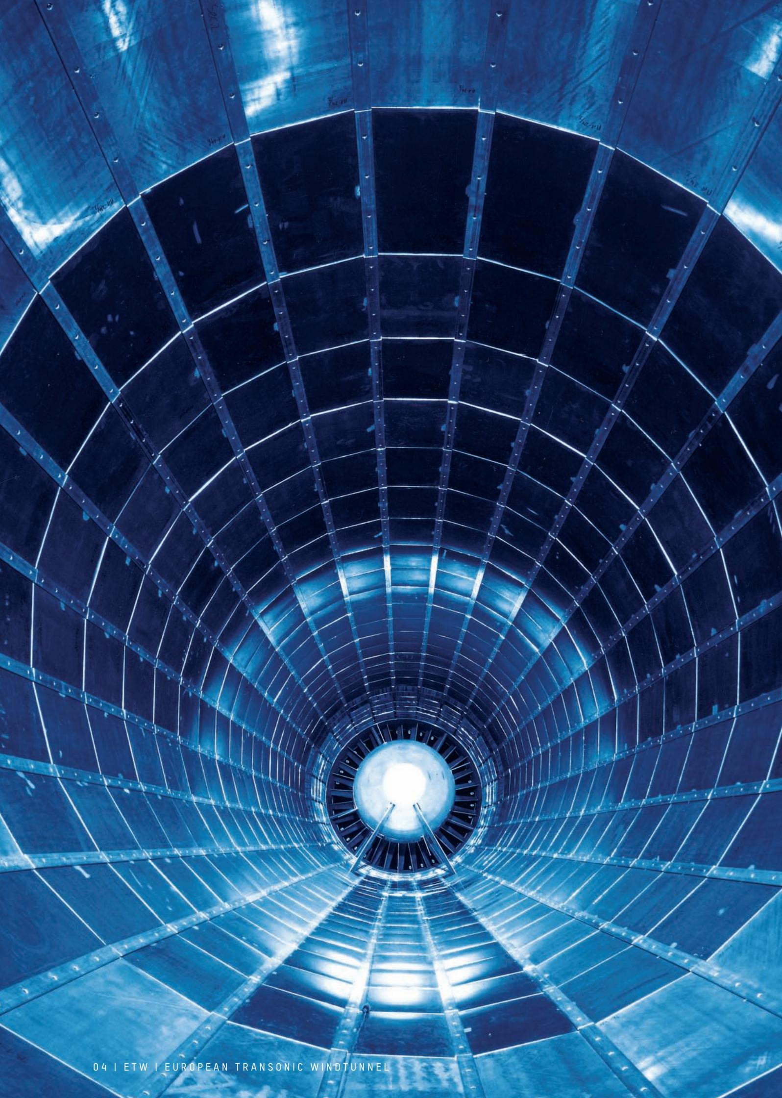
1. ETW tests aircraft models at the actual flight Reynolds numbers of the full-scale aircraft.
