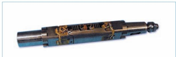
High-precision balances for full-span models
