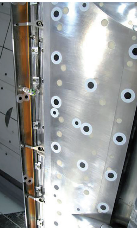
Detailed views of the SPT markers on the lower side of the wing and Krüger flap
