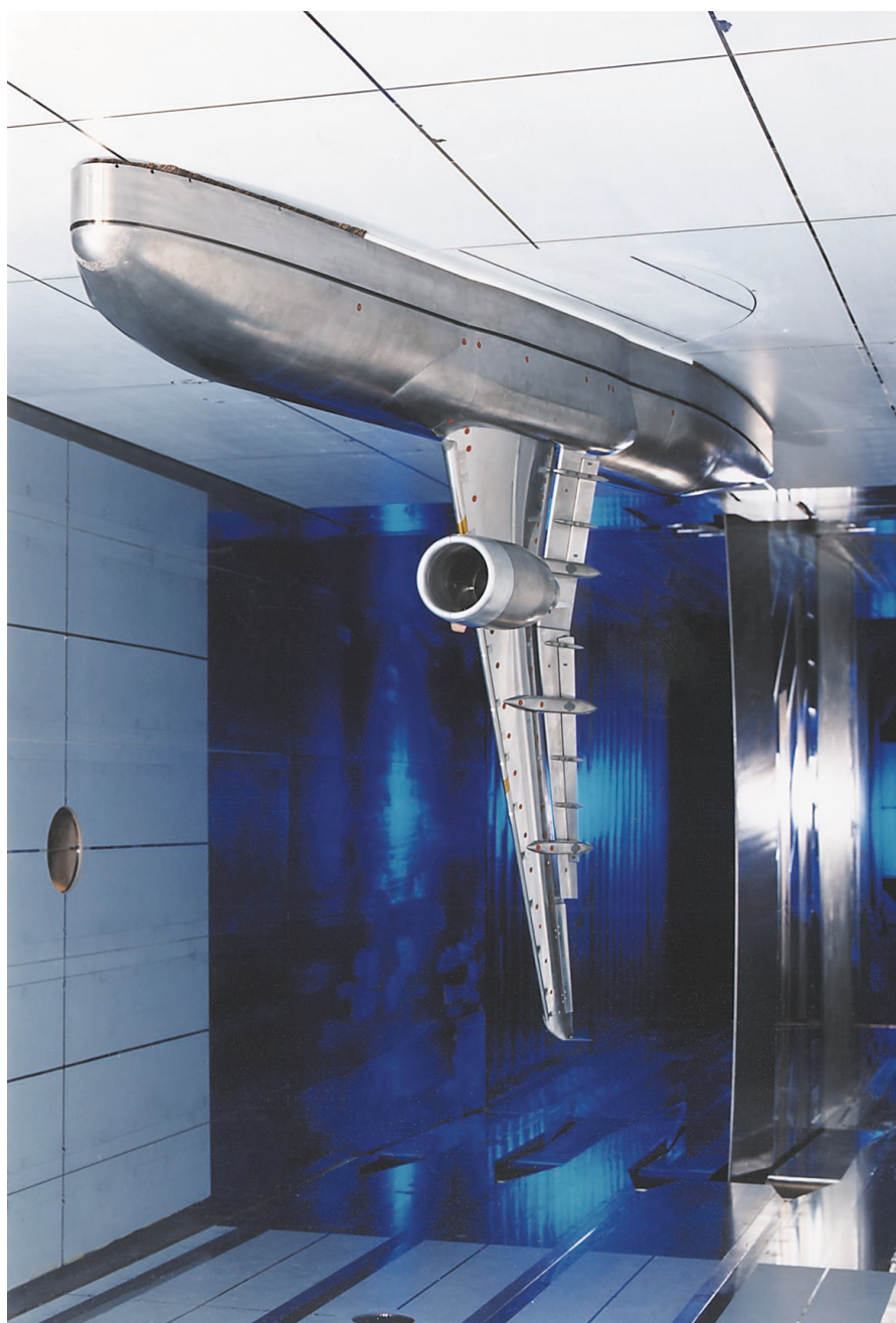
DaimlerChrysler Aerospace Airbus Half Model in the ETW Test Section
