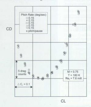
The optimum condition for standard 6 component testing has been determined to be the continuous model traverse mode at  $0.15^{\circ}$ /sec with a data acquisition rate of 5 Hz.
