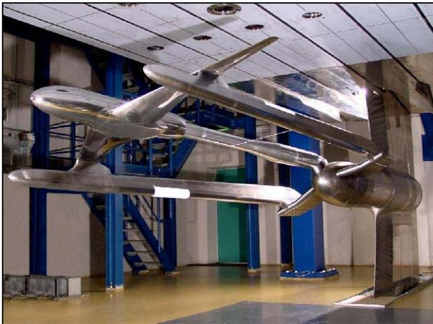
Figure 18 Model installed on the twin sting rig
