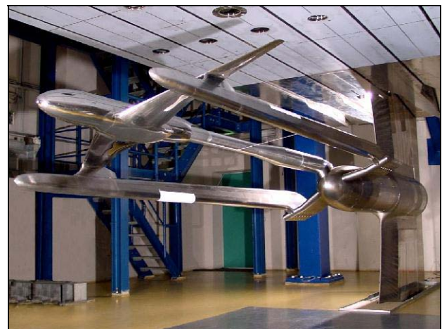
Figure 18 Model Installed on the Twin Sting Rig
