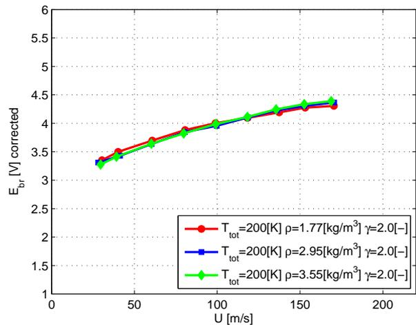
Fig. 20. Density influence at  $T_{tot} = 200[\text{K}]$  corrected
