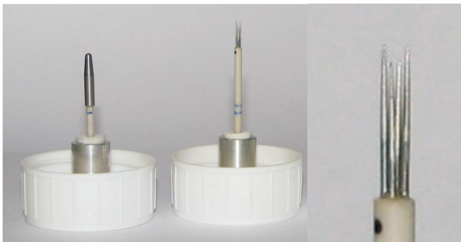
Fig. 1. DANTEC shortcut probe (left) and x-wire sensor (right and zoom)
