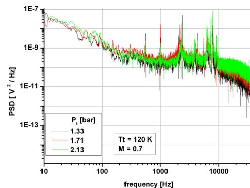
Fig. 46. Frequency spectra for varying density
