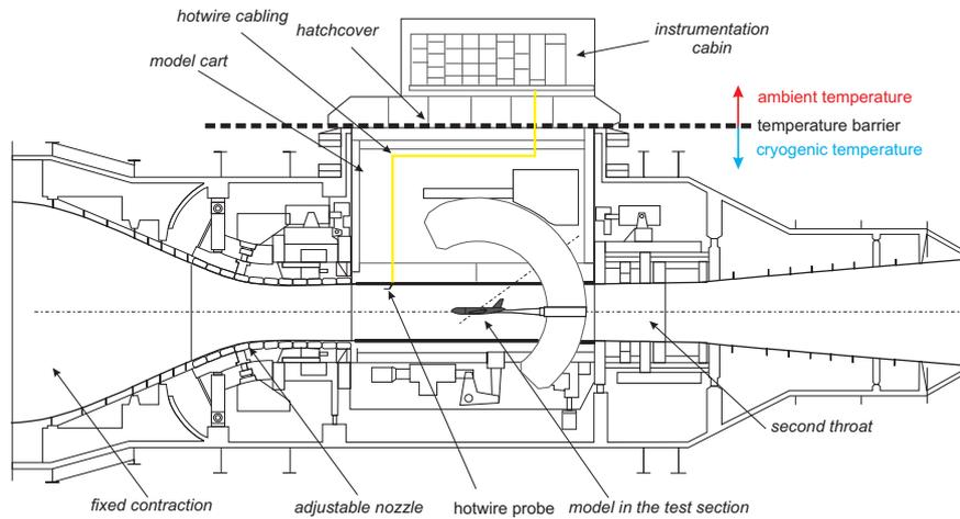
**Fig. 6. ETW side view with model cart**
