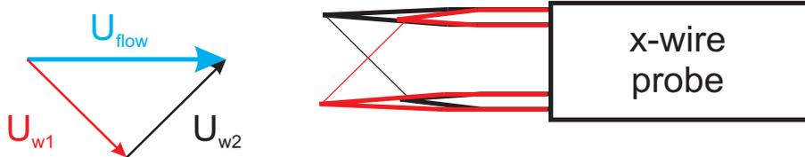
**Fig. 7. x-wire probe layout and used velocity definition**
