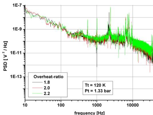
Fig. 47. Frequency spectra for varying overheat ratio
