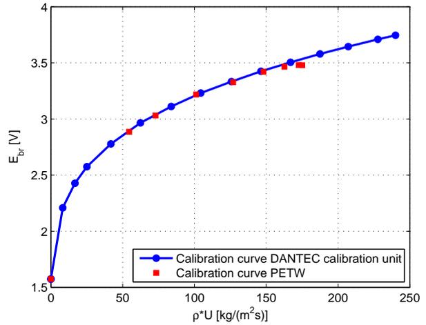
Fig. 14. Comparison of bridge output over mass flow
