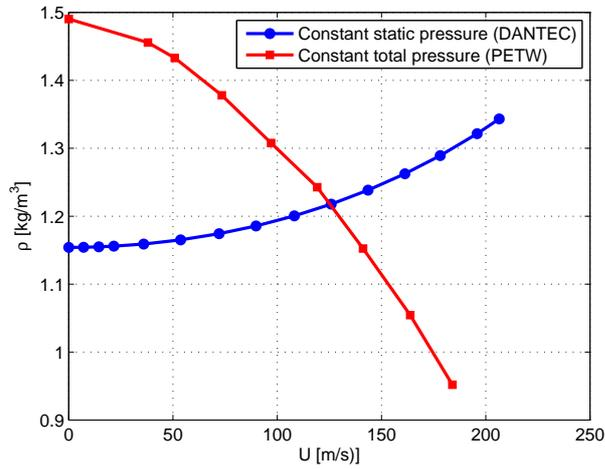
Fig. 13. Comparison of density characteristics over velocity
