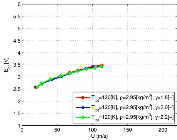
Fig. 28. Overheat ratio corrected  $T_{tot} = 120$ [K]
