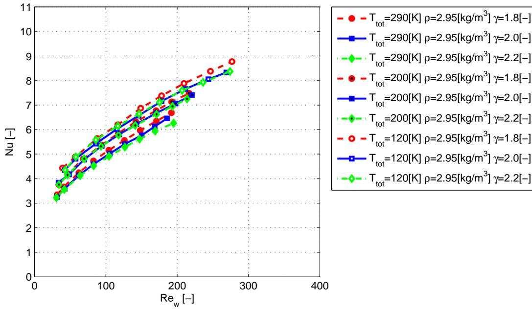
Fig. 35. Nusselt number over Reynolds number for different temperatures and overheat ratios
