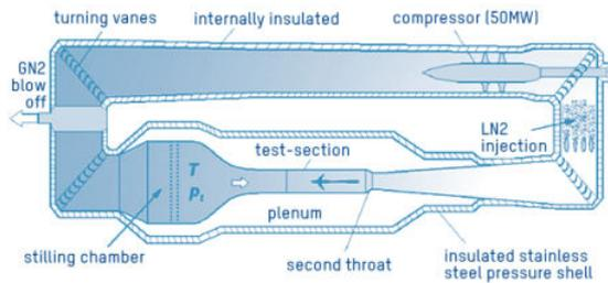
Fig. 2. ETW aerodynamic circuit
