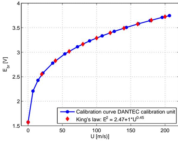
Fig. 11. Calibration results DANTEC calibration unit
