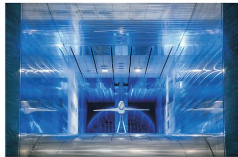
Fig. 3. Full model in ETW test section
