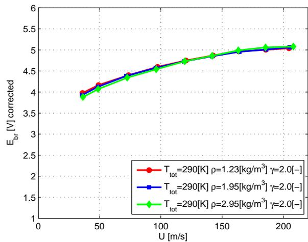
Fig. 18. Density influence at  $T_{tot} = 290[\text{K}]$  corrected
