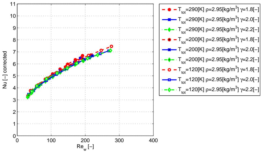
Fig. 43. Nusselt number over Reynolds number for different temperatures and overheat ratios
