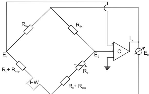
**Fig. 8. Anemometer bridge layout**
