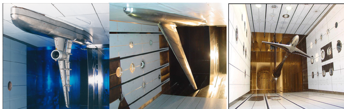
Figure 3: Test section configurations of ETW: solid (left), slotted side-walls (centre) or slotted top/bottom walls (right).
