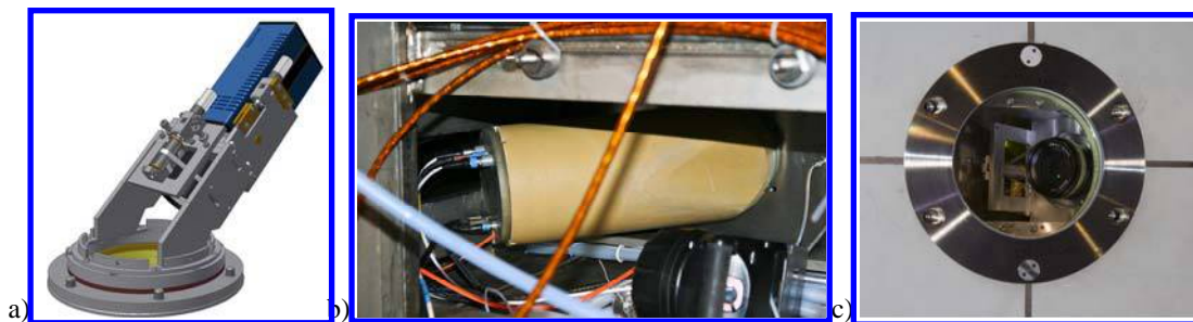
Figure 6. a) Sketch of opened camera module b) installation of angled housing viewed from the rear side of the test section c) camera lens behind test section window (as seen from inside).
