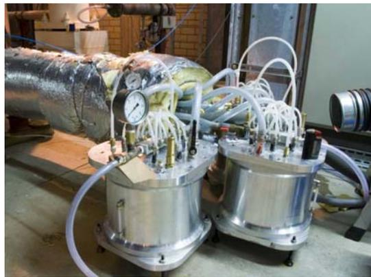
**Fig. 3:** Ice particle seeding system at ETW showing the DLR Laskin droplet generators for high volume rates and high operation pressures
