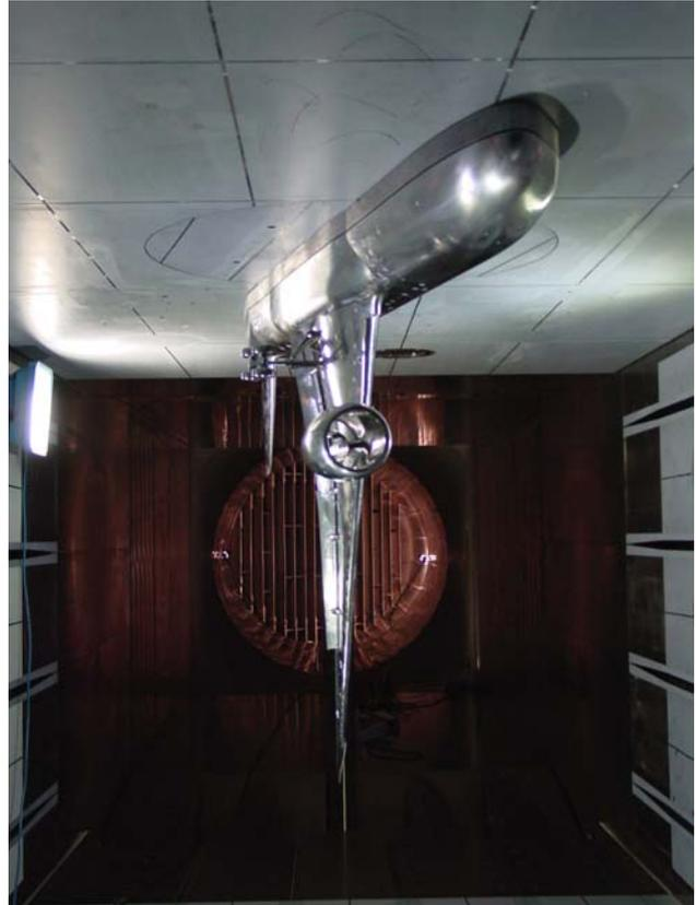
**Fig. 1.** 787 half model in ETW test section
