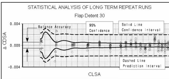
**Fig. 15.** Statistical analysis of landing  $C_D$
