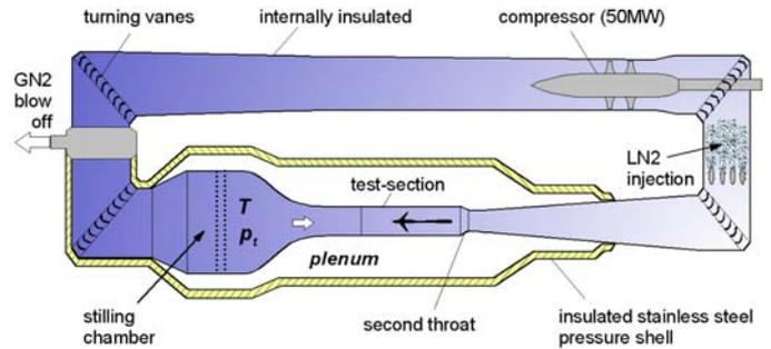
**Fig. 3.** ETW tunnel circuit
