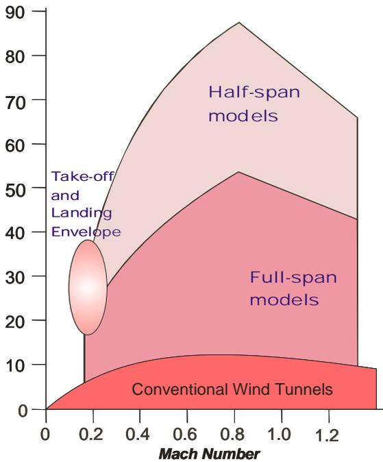
**Fig. 2.** ETW testing envelope
