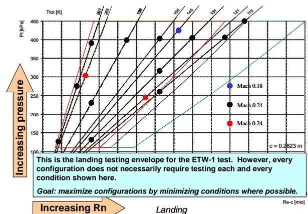
Fig. 8. Complete landing testing envelope
