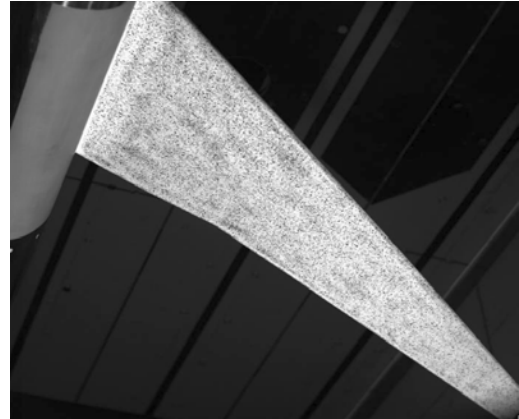
Figure 5. IPCT dot pattern on the wing of a cryogenic wind tunnel model tested in ETW.
