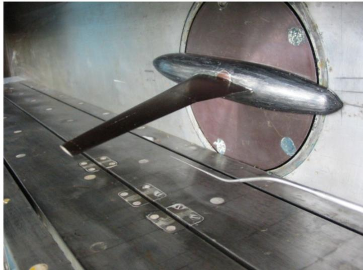
Figure 3: Half-model in T-125 wind tunnel.
