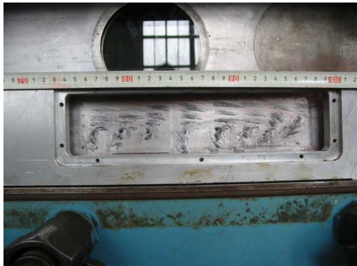
**Figure 10: Empty test section. Oil visualization. Slot flow pattern (after run).**
