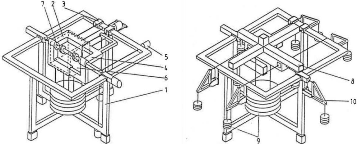
**Fig. 2 Schematic description of the Balance Calibration Machine [4].**
