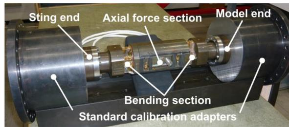
Fig. 4 ETW's B005 strain-gauge balance.
