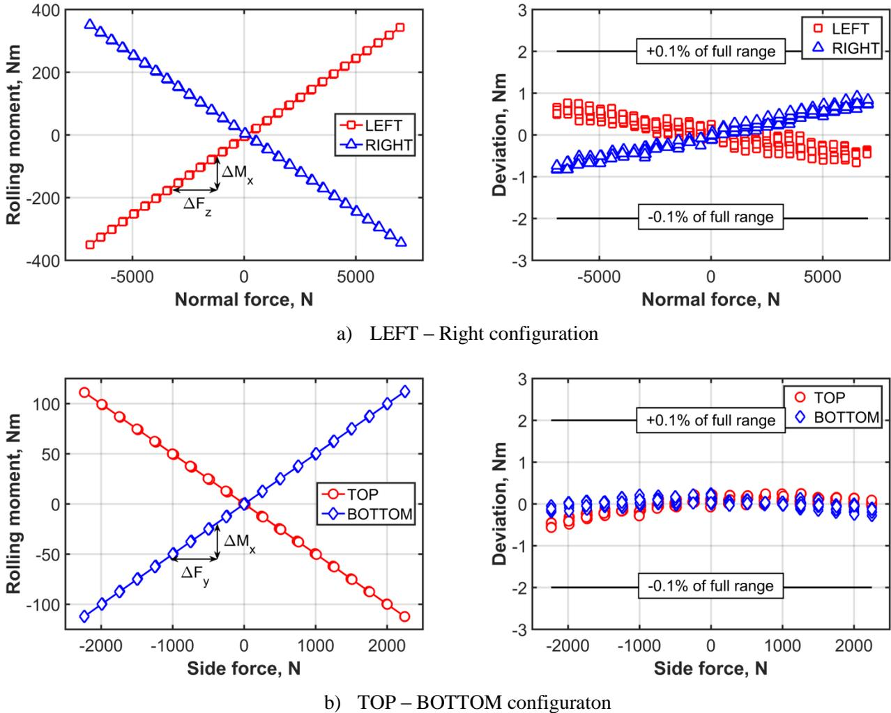
**Fig. 13 Results for rolling moment verification.**
