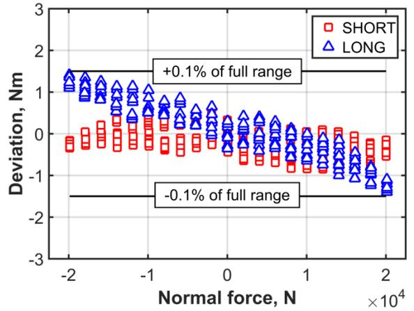
Fig. 14 Results for pitching moment verification
