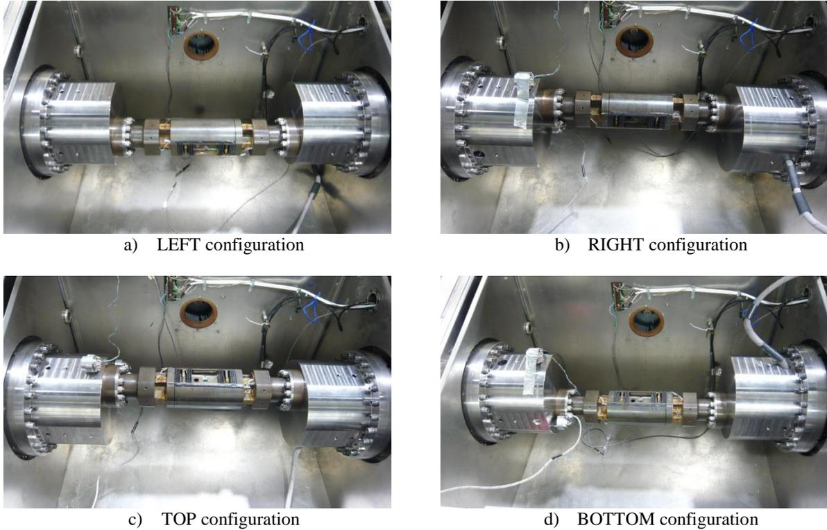
**Fig. 9 Installation of Lateral Offset Adapters.**
