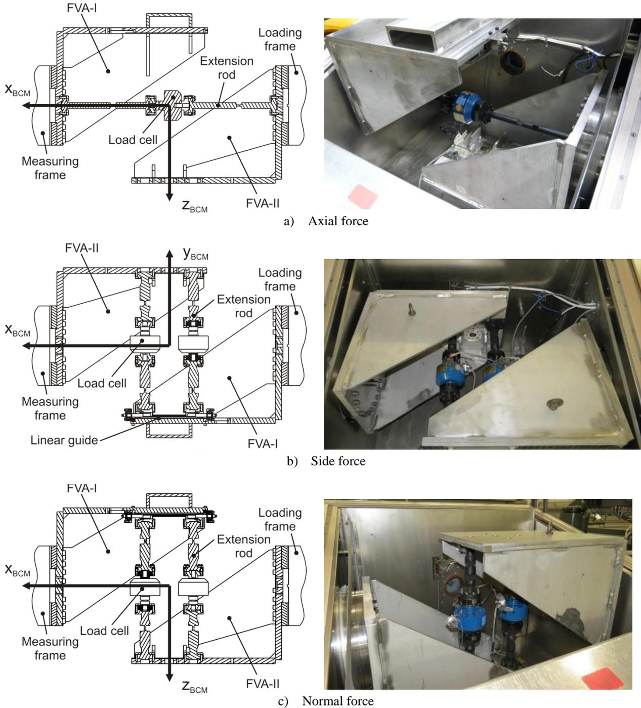
**Fig. 3 Adapter assemblies for force verification procedure.**
