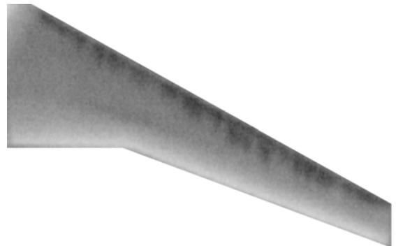
**Figure 3. Example of transition detection with the infrared imaging technique on a full model**
