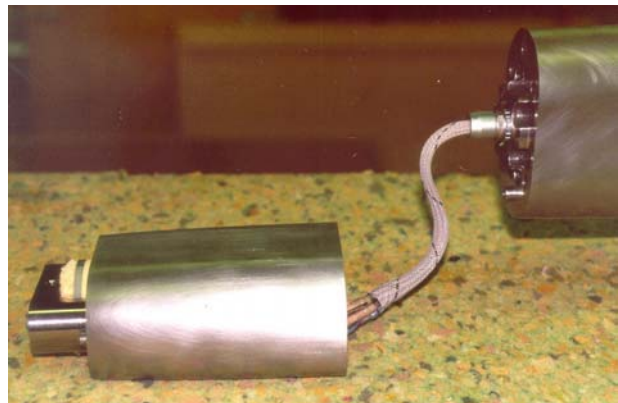
Figure 8: Boom Balance Inclinometer Housing
