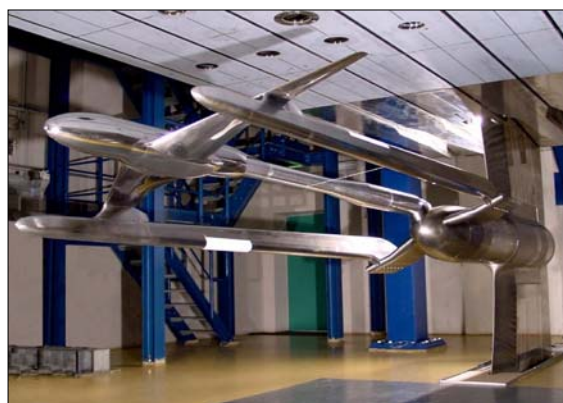
Figure 1: Model Installed on the ETW Twin Sting Rig
