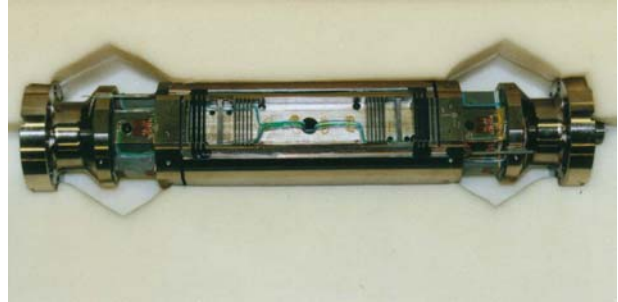
Figure 7: Split Fuselage Balance
