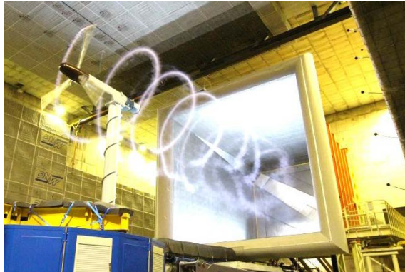
The “New-Mexico” wind turbine TNA test at the DNW-LLF test section. Photo: DNW.
