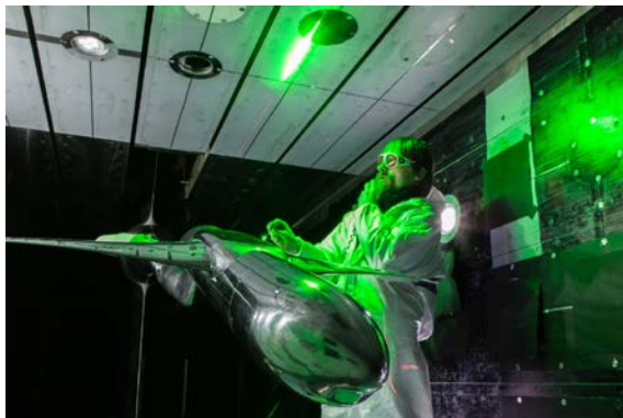
Adjusting PIV (Particle Image Velocimetry) for testing the NASA CRM during the ETW TNA. Photo: DLR.
