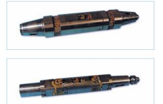
High-precision balances for full-span models
