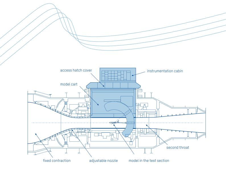
Model Cart with model in the test section
